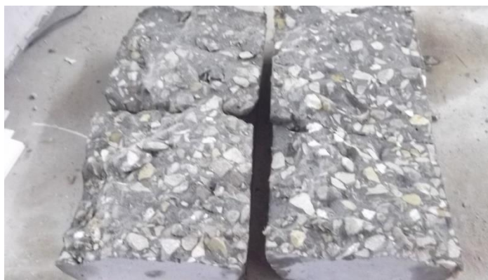
Figure 4-14: Splitting Tensile Strength Tests Results for Plain Concrete.
