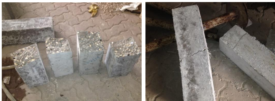
Figure 4-20: The mode of failure for flexural strength specimens.
