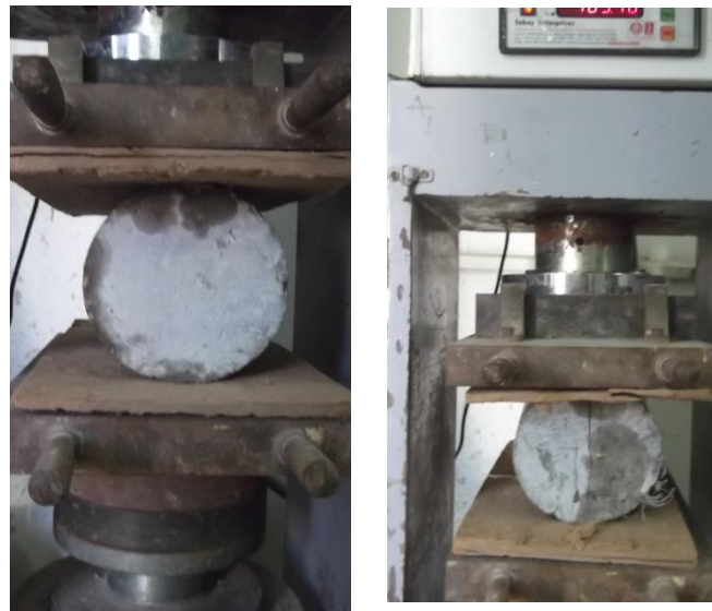
Figure 3-7: A typical setup of indirect tensile test.
