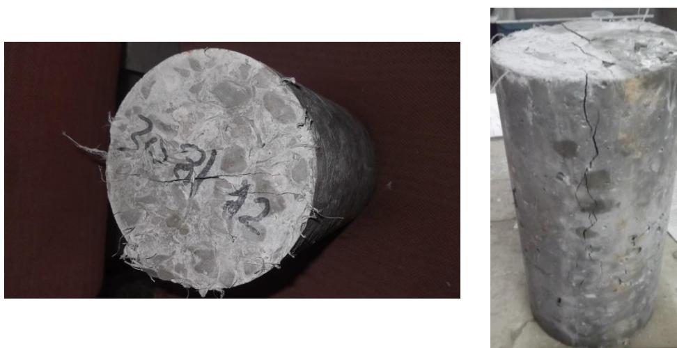
Figure 4-15: Splitting Tensile Strength Test Results for FR Concrete.
