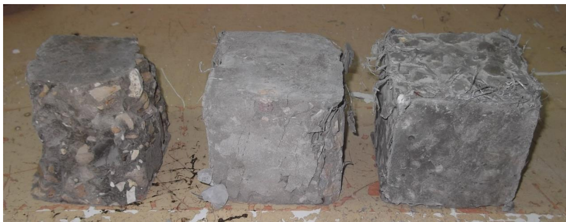
Figure 4-10: The mode of failure for compressive strength specimens.
